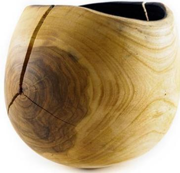
Fig 5: A cracked bowl made from green wood.
