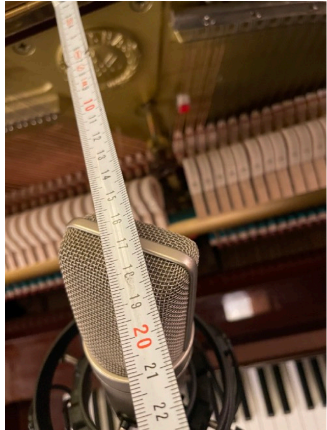
Fig.5 - The distance of the Neumann U87s from the piano's soundboard during recording.
