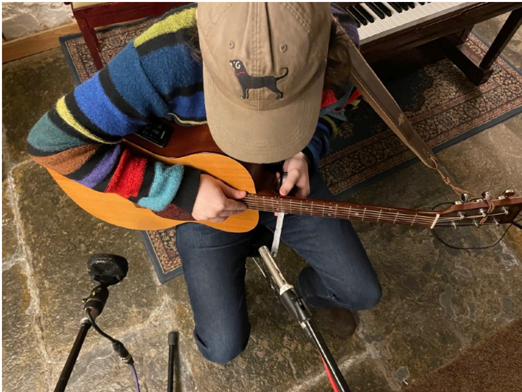
Fig.3 - The positioning of the AKG 451(right) and Coles 4038 (left) microphones during the recording of the acoustic guitar.
