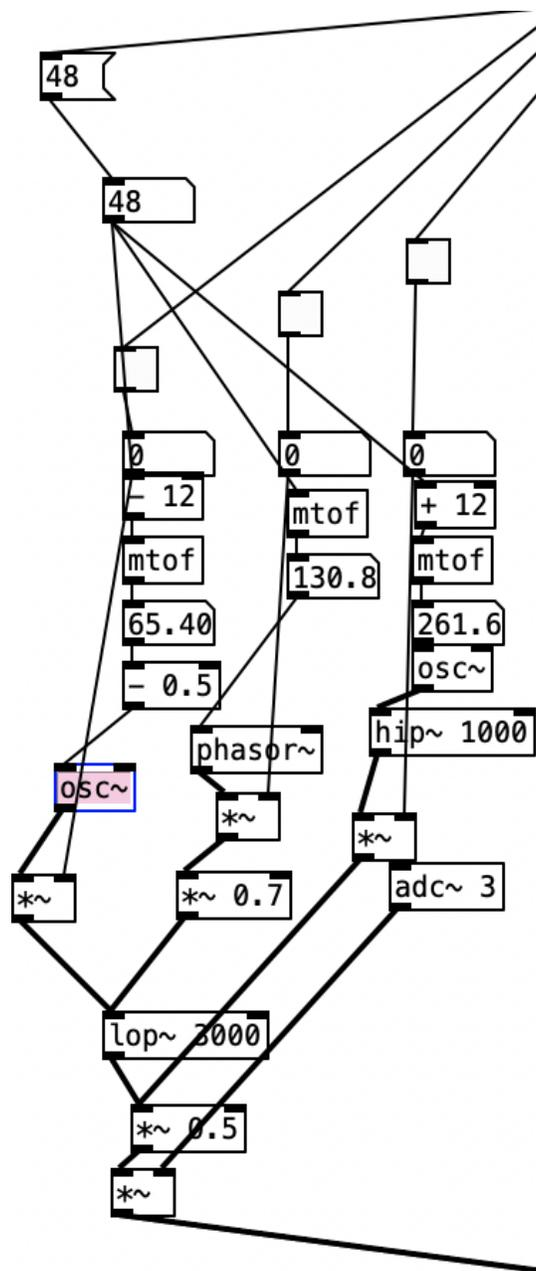
Fig.4. code from a single set of oscillators
