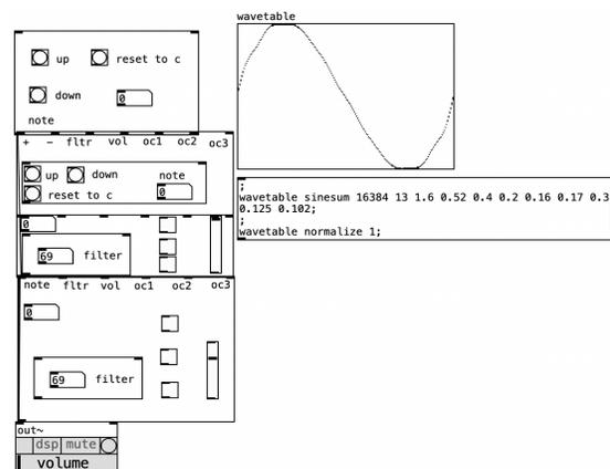
Fig.3, Wavetable synthesiser
