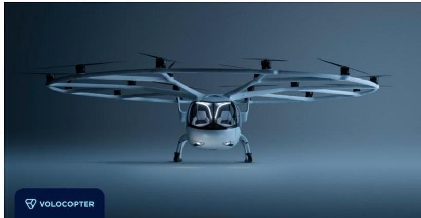
Fig. 30 VoloCity electric vertical take-off and landing urban mobility vehicle.
