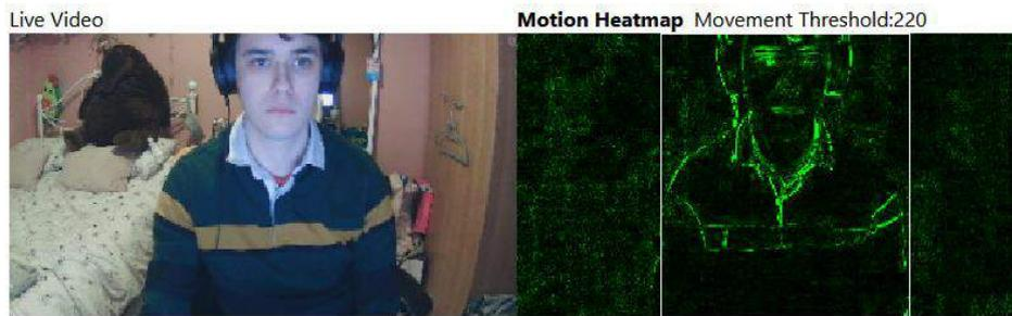
Figure 47 - Streaming video from NodeJS Livecam to the React canvas, which a modified DiffCamEngine evaluates for motion.
